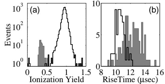
Figure 2. Discrimination of background events in the energy range 10–100 keV as demonstrated with CDMS II calibration data [6] from sources of photons (unfilled histograms) and neutrons (filled histograms). (a) Discrimination of photons is  $> 99.97\%$  efficient, limited by statistics. (b) Applying a cut based on phonon risetimes can remove  $> 97\%$  of the low-ionization-yield events (mostly electrons) while keeping  $> 50\%$  of the neutron events.
