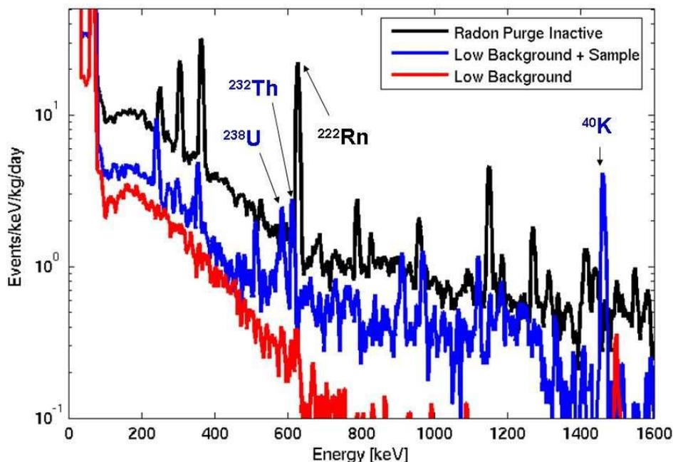
**FIGURE 1.** SOLO data taken using the 0.6 kg HPGe “Diode M” detector. From top to bottom: data taken without the Radon gas purge active, background data taken with a screening sample present (Hamamatsu R9288 PMTs) plus Rn purge, and background data (no sample) with Rn purge active.
