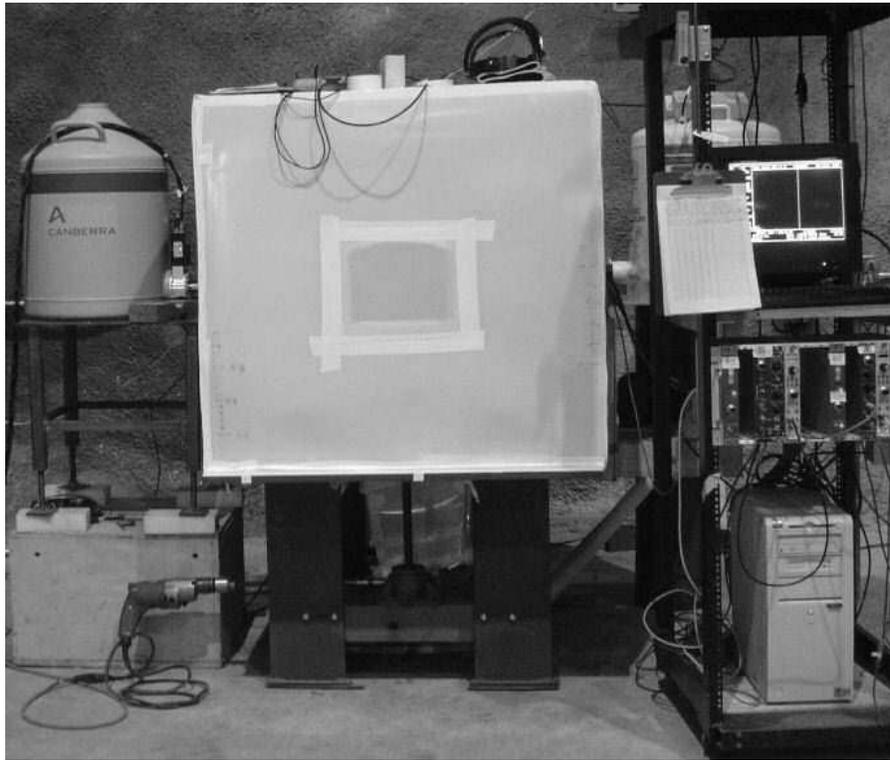
**FIGURE 3.** SOLO Gamma Screening Facility at Soudan Mine, MN. The Pb shield is surrounded by white mylar providing a Rn barrier. The LN dewars of the two HPGe detectors can be seen to the left and right of the main shield.
