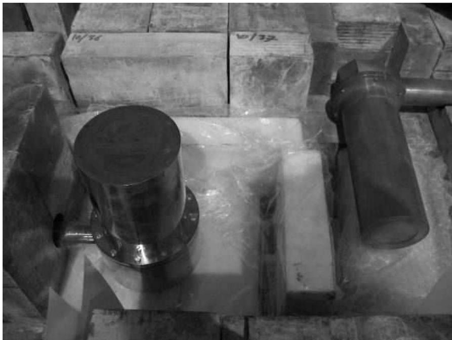
**FIGURE 4.** The two HPGe detectors on the ends of their Cu cold fingers can be seen, during shield assembly.
