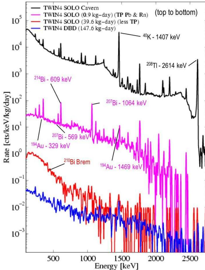
**FIGURE 2.** SOLO data taken with the TWIN detector. From top to bottom: cavern background rates, initial spectrum including TP brick, final spectrum without TP brick, and background taken during Double-Beta operation at Homestake.
